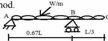
3. Using conjugate beam method, obtain the slope and deflections at A, B, C and D of the beam shown in fig. take  $E = 200\text{GPa}$  and  $I = 2 \times 10^{-2} \text{ m}^4$ .
