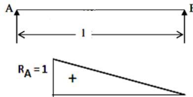
9. Sketch the influence line diagram for shear force at any section of a simply supported beam.
