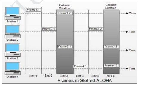
• In slotted ALOHA, if any station is not able to place the frame onto the channel at the beginning of the slot *i.e.* it misses the time slot then the station has to wait until the beginning of the next time slot.
