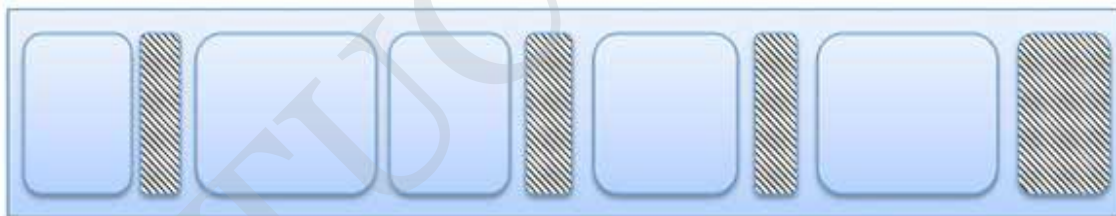
Fragmented memory before compaction
