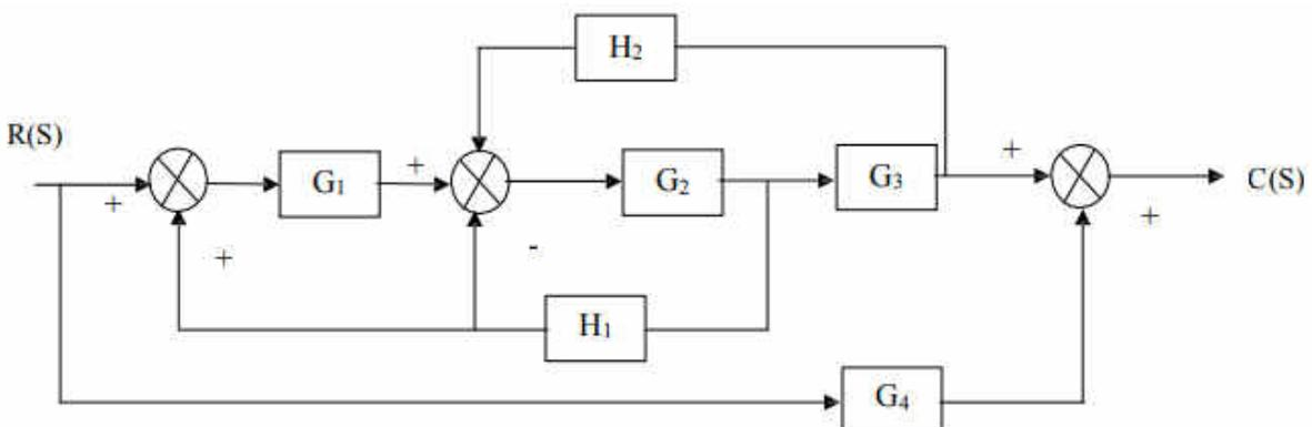
10. Find the overall gain  $C(s) / R(s)$  for the signal flow graph shown below.
