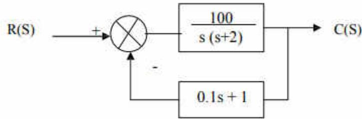
8. . A positional control system with velocity feedback is shown in fig. What is the response  $c(t)$  to the unit step input. Given that  $\zeta = 0.5$  and also calculate rise time, peak time, Maximum overshoot and settling time.
