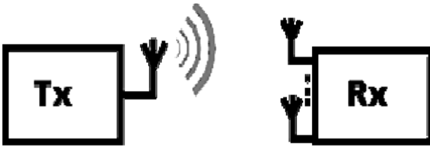
Fig. 4.7 SIMO - Single Input Multiple Output
