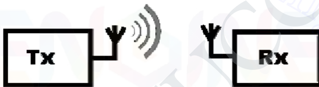
Fig. 4.6 SISO - Single Input Single Output
