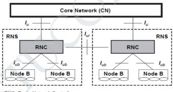
RNC: Radio Network Controller RNS: Radio Network Subsystem
