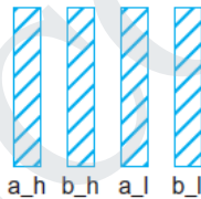
FIGURE 9.32 Reducing coupling noise on dual-rail busses
