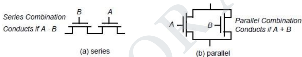
Figure 3 NMOS logic rules — series devices implement an AND, and parallel devices implement an OR.
