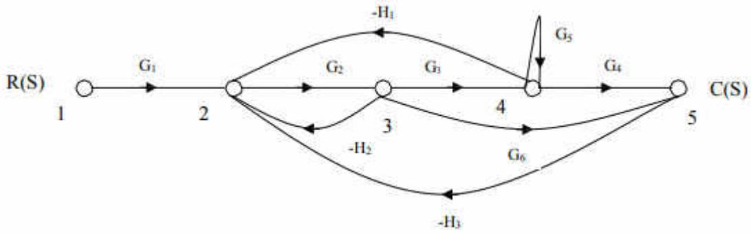
11. Find the overall gain of the system whose signal flow graph is shown in fig.
