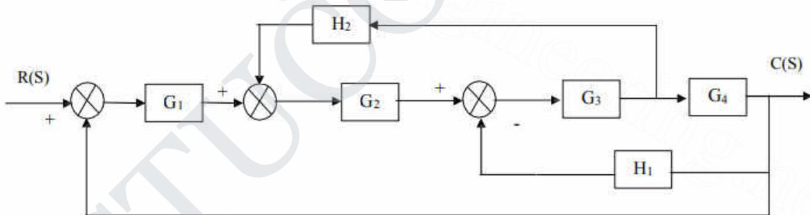
9. Obtain the closed loop transfer function  $C(S)/R(S)$  of the system whose block diagram is shown in fig.
