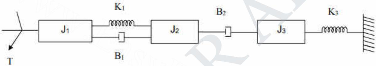
8. Determine the overall transfer function  $C(S)/R(S)$  for the system shown in fig.
