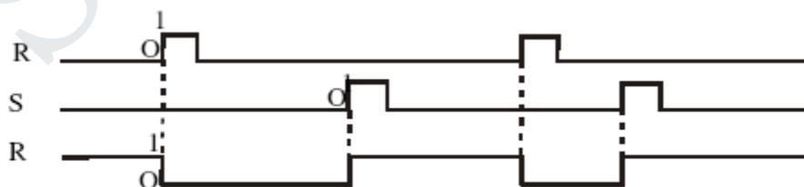
**Here the latch input has to be pulsed momentarily to cause a change in the latch output state, and the output will remain in that new state even after the input pulse is over.**
