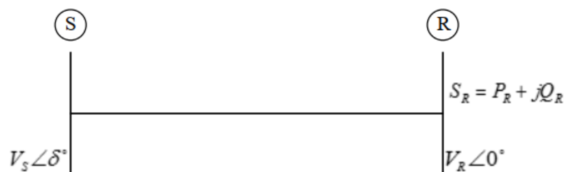
FIG.- TRANSMISSION LINE POWER FLOW
