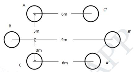
9. If the double circuit 3-phase line in Fig. has conductors of diameter 2.5 cm and distance of separation (D) is 2m in the hexagonal spacing arrangement, calculate the phase-to-neutral capacitance in μF per 100km of the line. **APRIL/MAY 2015 (R8)**
