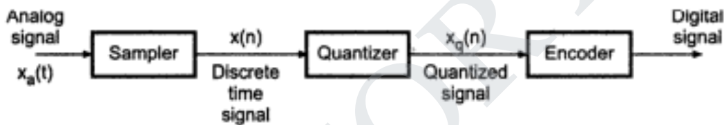
Basic block diagram of A/D converter
