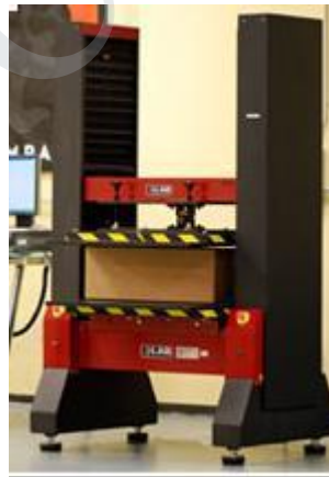
Compression tester for shipping containers
