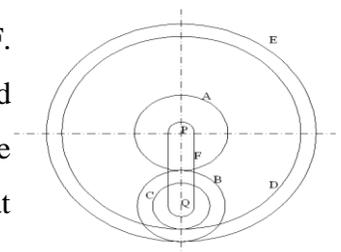
8. An epicyclic gear train as shown in figure is composed of a fixed annular wheel A having 150 teeth. The wheel A is meshing with wheel B which drives wheel D through an idle wheel C, D being concentric with A. The wheels B and C are carried on an arm which revolves clockwise at 100 rpm about the axis of A and D. If the wheels B and D have 25 and 40 teeth respectively, determine the number of teeth on C and speed and sense of rotation of wheel C.
